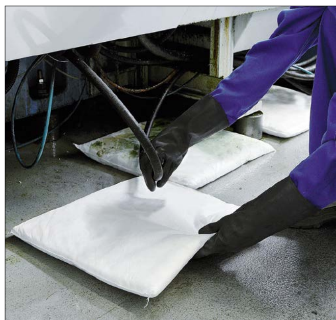
Cushions for collecting dripping oil from machinery
