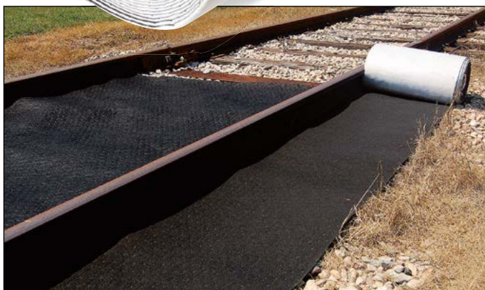
Use on railway lines: the wide roll fits snugly between the rails. Side areas are protected with the narrow roll.
