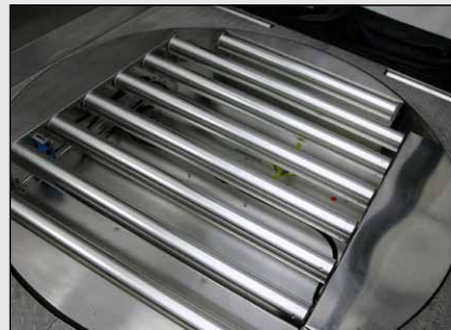
Pallet turntable , heavy duty stainless steel turntable set into the floor; controlled by the HMI screen in the inner room and connected to the main conveyor system.
