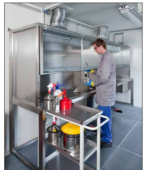
Compact Work bench for paint mixing and paint work, built into a fire-rated DENIOS WFP container.
