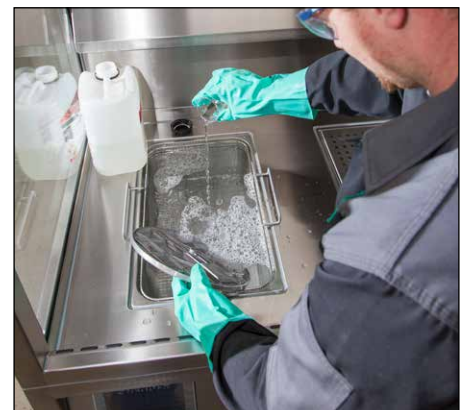
Ultrasonic tank incl. temperature control
