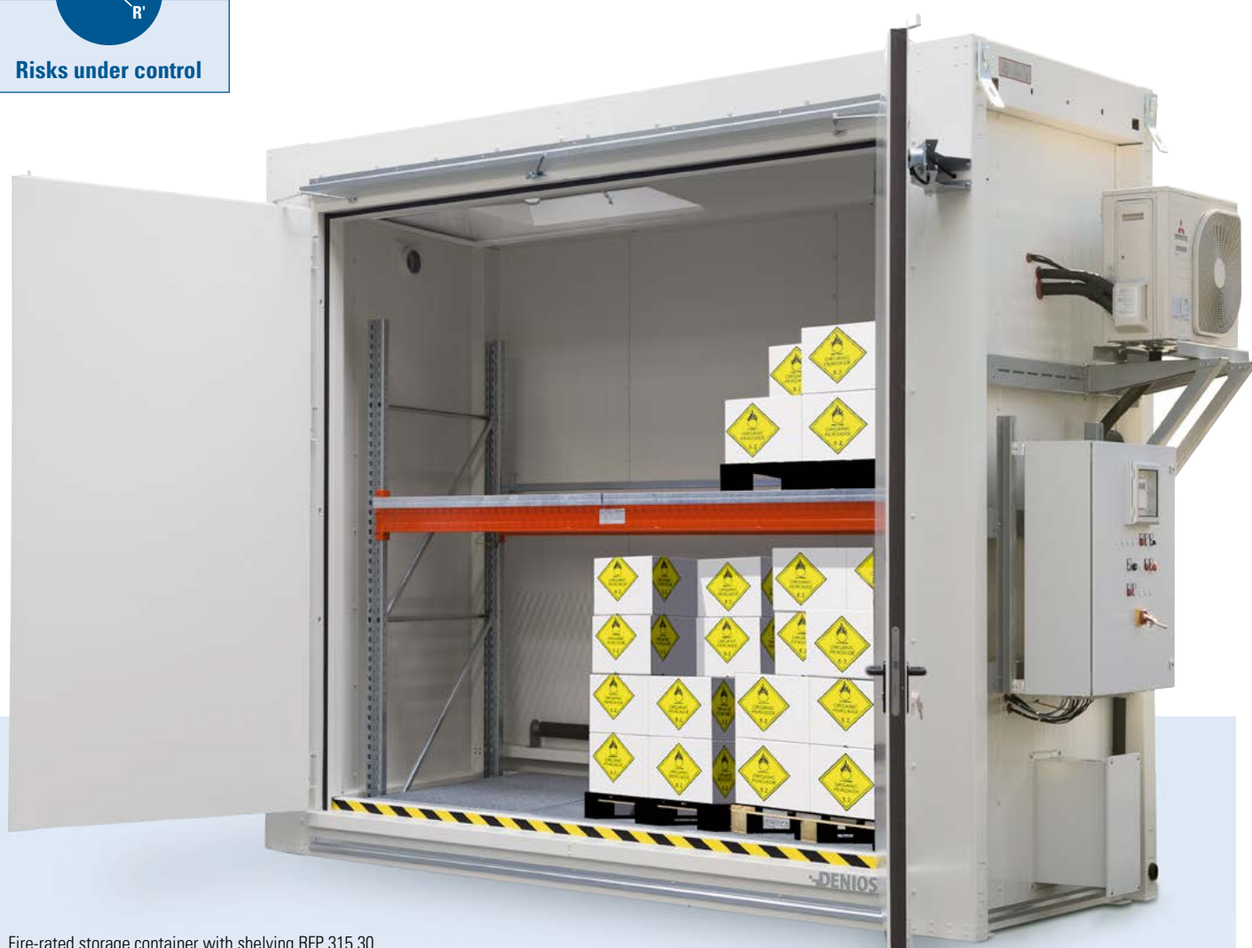
Fire-rated storage container with shelving RFP 315.30 with climate control, fire protection F 90 (REI 90) and pressure relief device in the roof
